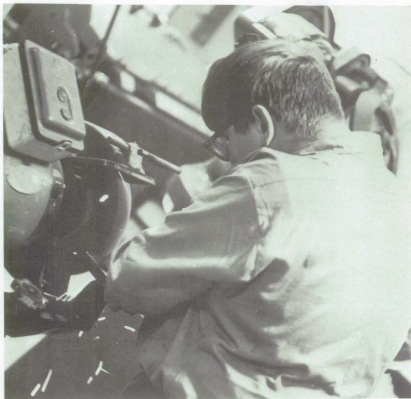
A student of Welding-Sheetmetal class at the Vo-Ed school smooths the weld by grinding.
