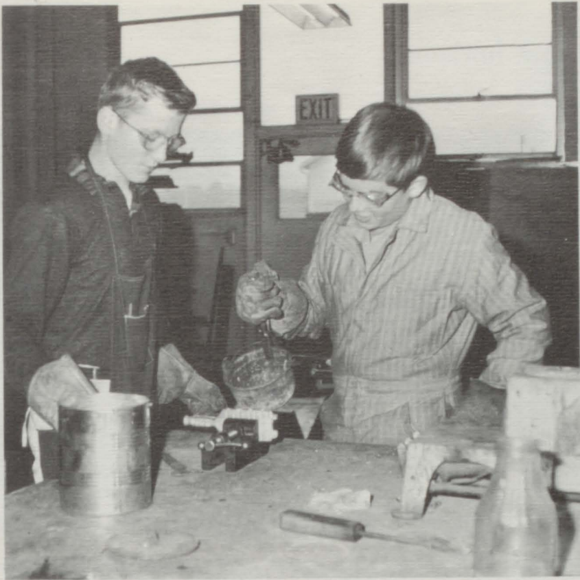
Gary Ford aids Joe Passerell in pouring molten metal into a mold.
